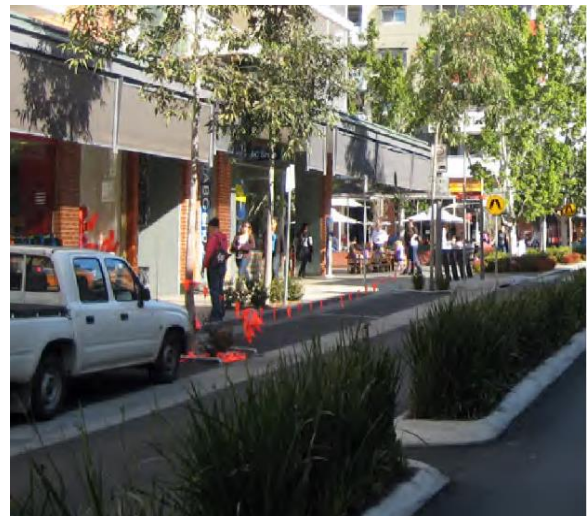
Photo 4.2. Awnings cover the footpaths but do not encroach beyond alignments of existing street kerbs and accommodate street tree plantings where appropriate.
