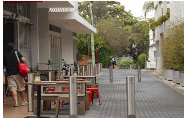
Photo 5.4. Shared paths should have signage and surface treatments that clearly show that it is an environment shared by pedestrians and vehicles (where relevant).
